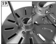
Remove 2 screws in yoke (see insert). Remove 3 screws with keyhole slots from top of fan.
